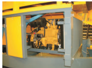
Diesel engine and Load Sensing hydraulic
