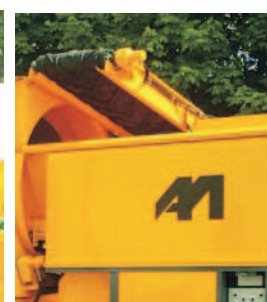
Discharge conveyors for the "fine" and "oversize" fractions with setting in position and hydraulic unfolding (optional conveyor, length: 5m)
