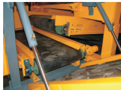
TR 1860, with foldable discharge conveyor for the fine fraction (optional equipment).
