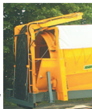
Discharge conveyors for the "fine" and "oversize" fractions with setting in position and hydraulic unfolding (optional conveyor, length: 5m)
