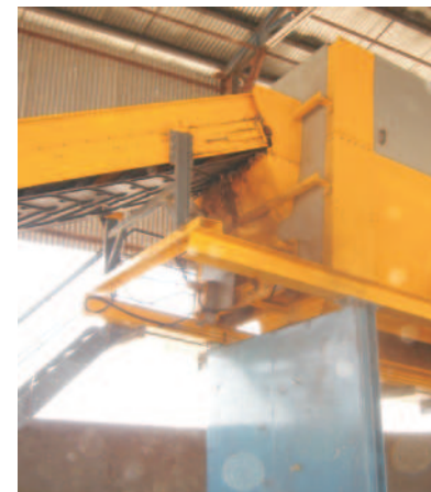
Photographs above: (1) the discharge point of the conveyor in the drum is designed to use the maximum of the sieving surface. (2) The robust drums are constructed from strong rectangular section tubing which makes a rigid frame, increases drum life and contributes to mixing and aerating the screened material. (3) Heavy industrial brushes are hinged to move with the drum and ensure permanent cleaning of the screen mesh.
