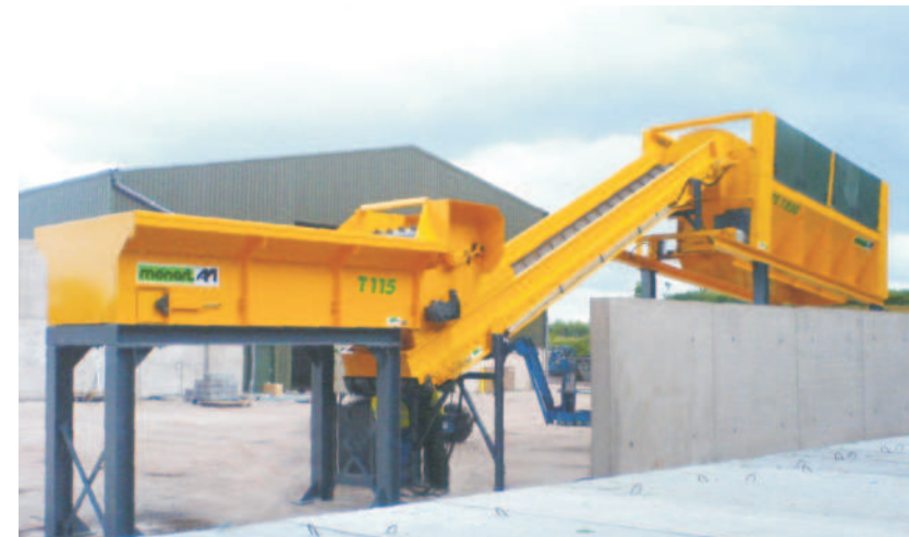
Basic equipment: hopper • conveyor • drum
