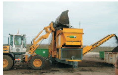
TR 1860, with foldable discharge conveyor for the fine fraction (optional equipment).
