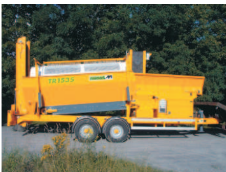
Highway chassis with double road axle, approved for 80 km/h, ABS braking with pneumatic control, rear bumper and cyclist side bumper, road lights and other equipment in conformity with the highway code. Wheels equipped with road tires 285/70 R 19.5
