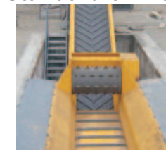
Some examples of Ménart "Tailor Made" installations: (1) client's own colours and double sized hopper with rubber belt conveyor, (2) hopper lower than ground level with an extra-long conveyor, (3) hydraulic drive rather than electric, (4) conveyer for the fine fraction under the drum, etc.
