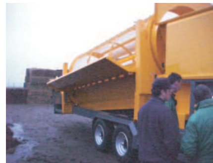
Conveyors for the fine fraction: • conveyor under the drum • transverse conveyor • foldable discharge conveyor
