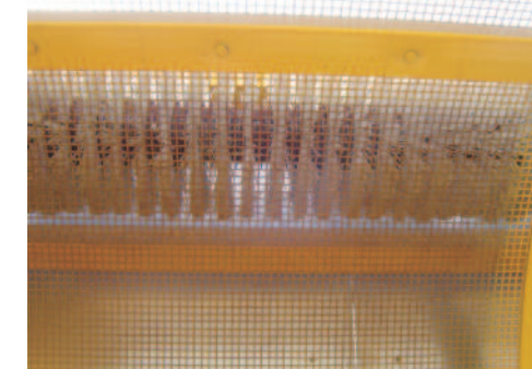
Photographs above: (1) the discharge point of the conveyor in the drum is designed to use the maximum of the sieving surface. (2) The robust drums are constructed from strong rectangular section tubing which makes a rigid frame, increases drum life and contributes to mixing and aerating the screened material. (3) Heavy industrial brushes are hinged to move with the drum and ensure permanent cleaning of the screen mesh.
