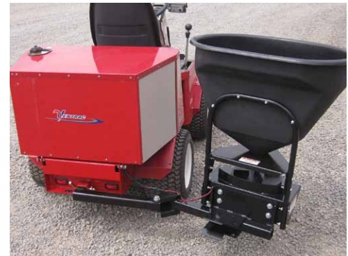
Mounting Bracket on the 3000 series swings out to give access to the engine.
